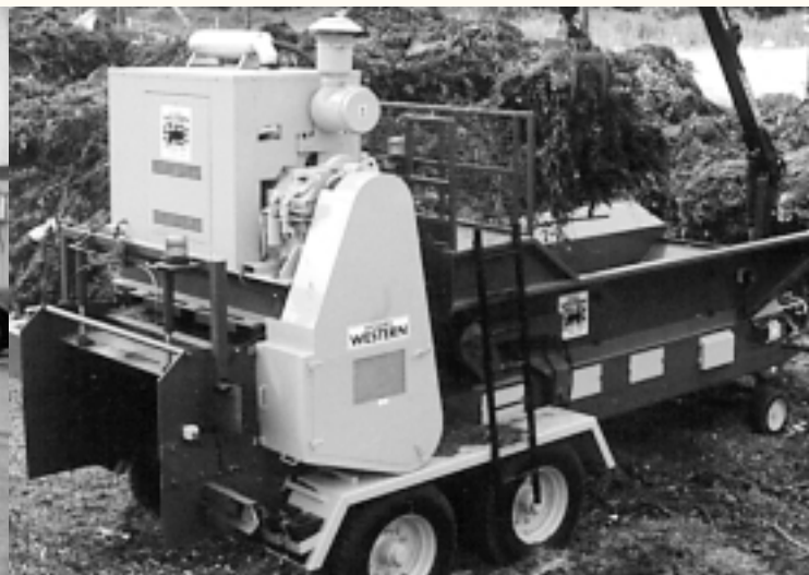
21 KPTO, WOOD CHIPPER 350 kW @ 1800 rpm
